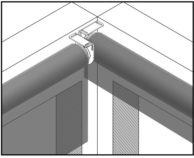
TYPICAL BUTT AND PASS WITH 1-1/4 to 1-1/2 +/- LIGHT GAP
