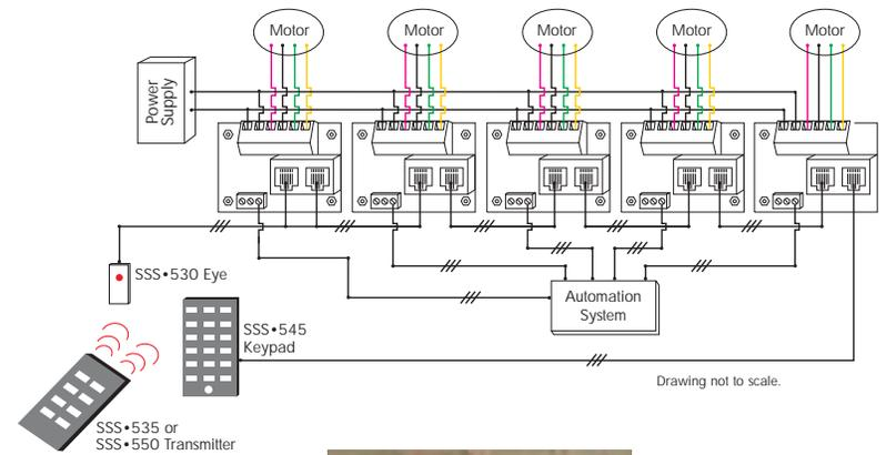
Our exclusive SSS-525 LouverLevel™ controller combines the latest technology with practical operation of our Solar Shading Systems Motorized Plantation Shutters. The controller operates via infrared commands from our transmitter or wall mounted keypad. The infrared codes are all learnable which allows any home automation system with
